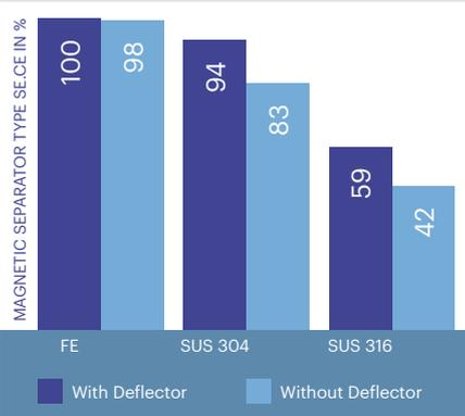
The **effectiveness graph** shows what you can expect from an Easy Cleanflow magnet. The idea is to allow you to enter product parameters so you can know for certain which particles will be captured. We utilize a computer simulation process in which we can change the parameters to match various products. These could be anything from milk powder to cocoa powder or even quartz sand. This enables us to make a prior assessment of the expected effectiveness of our magnetic separators.
